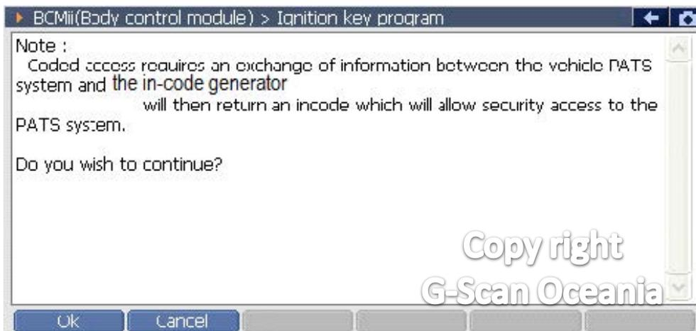
\*\* If not showing this screen, please IG off and take off the key for a 35 seconds. And retry first procedure.(G-scan must disconnect from the car)
